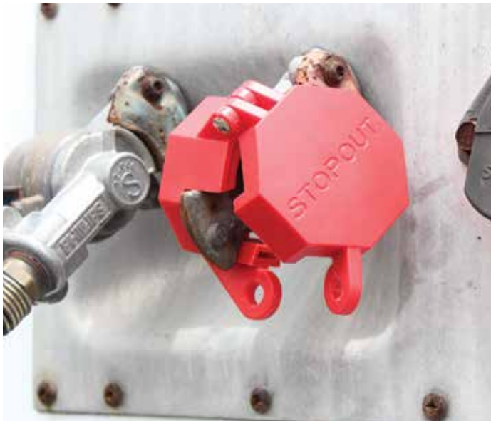
Close device over Glad Valve.
