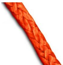
SuperMax II is an ultra high molecular weight polyethylene (UHMWPE), Dyneema® SK75 fiber braided rope. It offers the strongest tensile strength per weight available. This rope is stronger than wire rope of the same diameter, at 1/8 the weight. A special heat treatment enhances its anti-abrasion characteristics.
