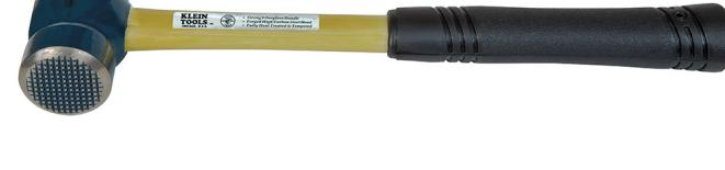
Klein Tools Lineman's Mill-Faced Hammer has one milled face for driving staples used in pole-line work and common, unhardened nails. The other face is smooth for driving heavier duty hardware.
